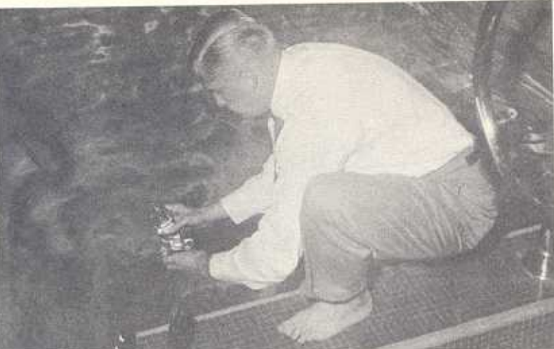
Collecting water sample for bacteriological analysis and chlorine test at swimming pool.
