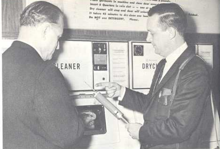
Engineer collecting sample in dry cleaning establishment to detect potentially dangerous gasses in the air.
