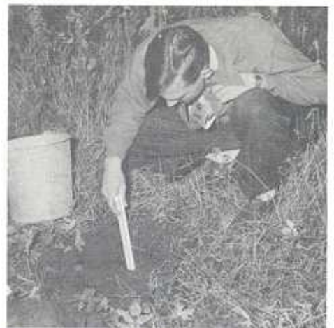
Testing the soil determines its ability to disperse septic tank effluent.
